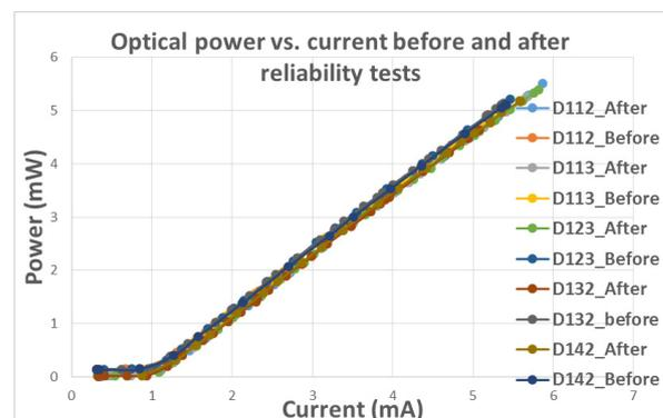
Figure 3: optical output power vs. current for one of the designs.
