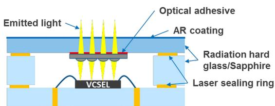
Figure 1: Schematic of one of the 3 stack designs.
