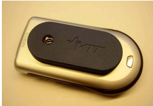
Fig. 35. Microscope lens system attached to a Nokia 6630 camera phone.
