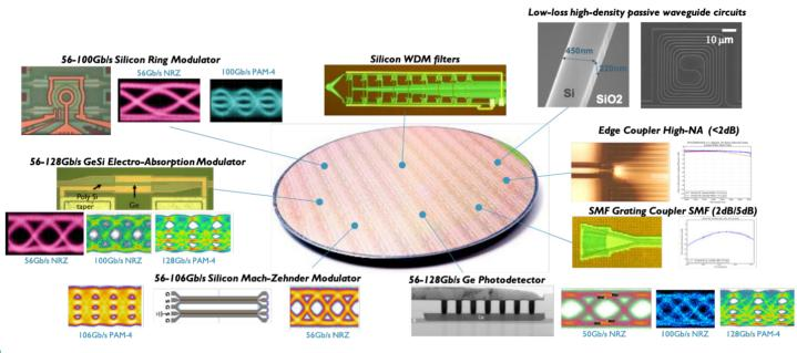
Imec's versatile 50G+ silicon photonics platform
