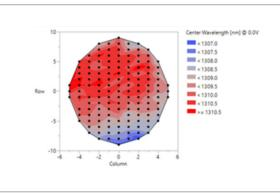
Microring Modulator Resonant WavelengthWafer-scale distribution (300mm, 1-  $\sigma$  = 0.9nm)
