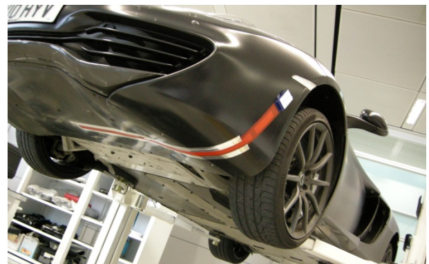
Figure 3: Pressure Strip applied to a sports car to measure front floor pressure suction.
