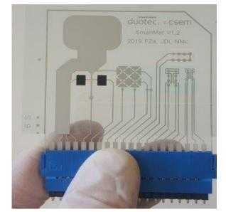
Figure 2: Pressure sensors (test features) for smart shelfs (Turck duotec case).
