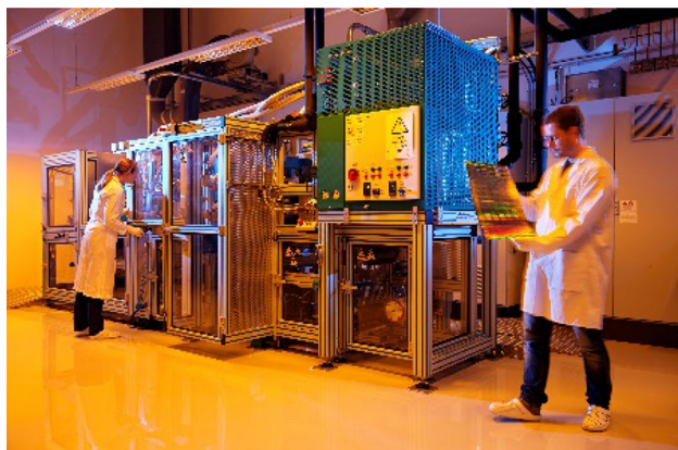
Fig. 1 The photograph of our roll-to-roll (R2R) UV Nanoimprint Lithography (NIL) pilot line
